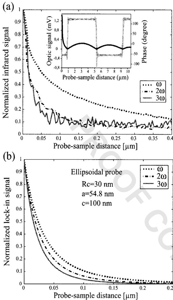
FIG. 3. (a) Experimental retract curves measured at  $\lambda = 10.6 \mu\text{m}$ . Inset: large-scale retract curve at  $\omega$ . (b) Calculated approach curves for an ellipsoidal tip with  $R_c = 30 \text{ nm}$ .
