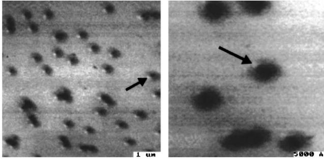
FIG. 6. Optical images recorded in the infrared with two different tips ( $\lambda = 10.6 \mu\text{m}$ , normal polarization). A bright spot is observed around each hole at a well-defined orientation indicated by the arrows.
