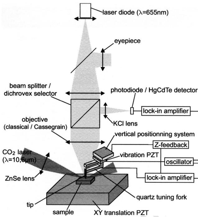
FIG. 1. Schematic view of both visible and infrared experimental setups.
