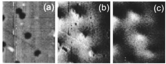
FIG. 4. Images obtained with a transmission mode ANSOM ( $\lambda = 780 \text{ nm}$ , scan size:  $2.5 \mu\text{m} \times 3 \mu\text{m}$ ). (a) Topographic image, (b) optical images recorded in tapping mode, that is, with the feedback loop active; and (c) in constant height mode, with the feedback loop disconnected and the tip slightly withdrawn.
