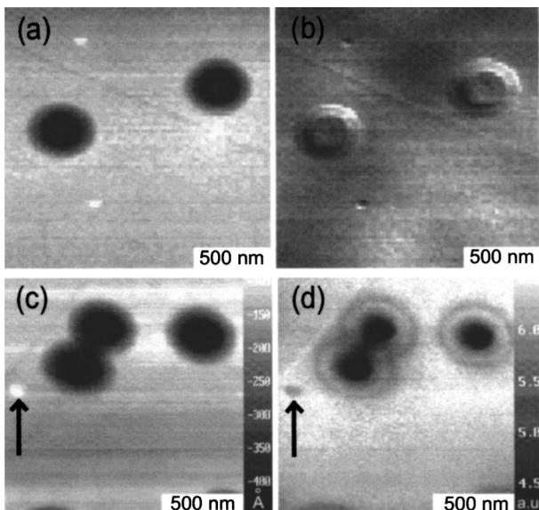
FIG. 2. (a) Topographic image. (b) Near-field image ( $\lambda = 655$  nm). (c) Topographic image. (d) Near-field image ( $\lambda = 10.6 \mu\text{m}$ ).
