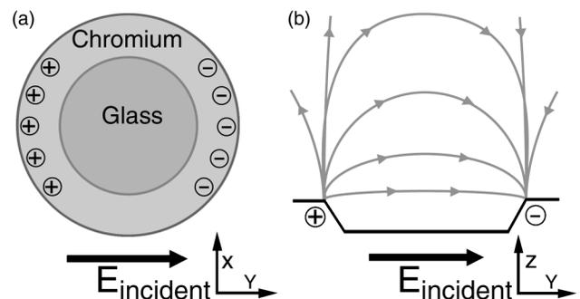
FIG. 5. (a) Distribution of surface charges around a hole under illumination. (b) Resulting stray field distribution.
